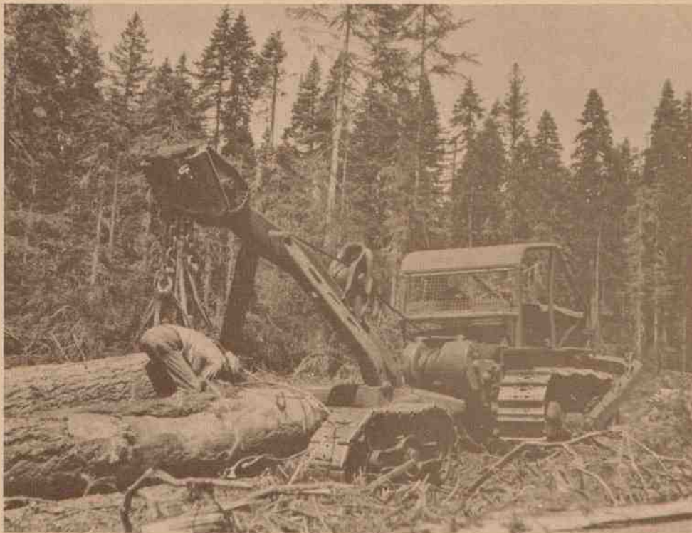
IV-18. A more substantial form of commercial forestry endeavor returned to the McLoughlin Unit during the 1940s and 1950s. This scene shows a tractor logging operation on the Daley Creek Timber Sale, 1953. The "cat-skinner" yards the logs by means of an "Athey-wheeled" Carco logging arch. (RRNF Collection)
